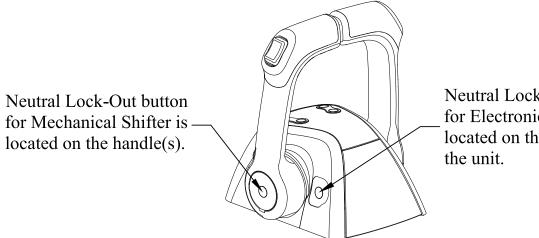
Neutral Lock-Out button for Electronic Shifter is located on the aft side of
