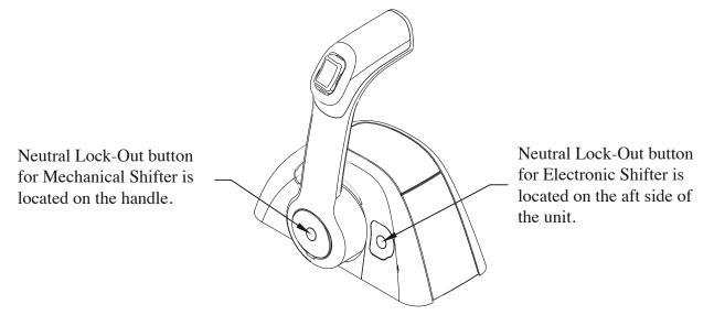
Reverse the shift mechanism to stop a boat that is moving forward. This change in direction will provide a "braking action" and slow the boat.
