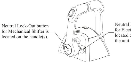
Neutral Lock-Out button for Electronic Shifter is located on the aft side of the unit.
