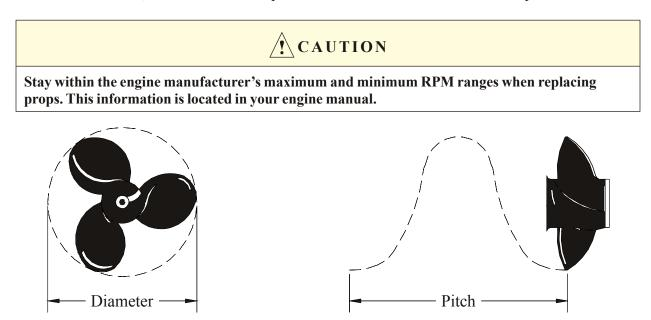
Diameter and pitch are the two basic dimensions of a propeller. Diameter is the distance across the circle made by the blade tips as the propeller rotates. Pitch is the theoretical (not accounting for slippage) forward distance the propeller would move in one revolution. An example of a propeller dimension would be 14 X 17 for a propeller having a diameter of 14" (35.6cm) and a pitch of 17" (43.8cm).
