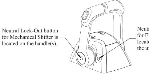
Neutral Lock-Out button for Electronic Shifter is located on the aft side of the unit.
