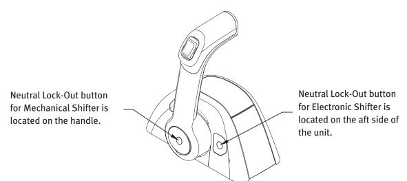
If your boat is equipped with Helm Master<sup>™</sup> there is a feature that is similar to a neutral lockout on other boats. When activated, the free throttle button allows opening the throttles on all engines without engaging the forward or reverse gear. The active indicator will be illuminated during operation. See Yamaha Helm Master<sup>™</sup> Operation Manual for detailed instructions.
