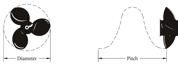
Diameter and pitch are the two basic dimensions of a propeller. Diameter is the distance across the circle made by the blade tips as the propeller rotates. Pitch is the theoretical (not accounting for slippage) forward distance the propeller would move in one revolution. An example of a propeller dimension would be 14 X 17 for a propeller having a diameter of 14" (35.6cm) and a pitch of 17" (43.8cm).
