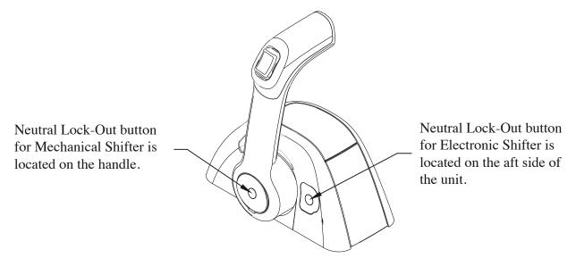
If your boat is equipped with Helm Master<sup>TM</sup> there is a feature that is similar to a neutral lockout on other boats. When activated, the free throttle button allows opening the throttles on all engines without engaging the forward or reverse gear. The active indicator will be illuminated during operation. See Yamaha Helm Master<sup>TM</sup> Operation Manual for detailed instructions.
