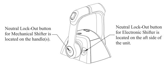
If your boat is equipped with Helm Master<sup>TM</sup> there is a feature that is similar to a neutral lockout on other boats. When activated, the free throttle button allows opening the throttles on all engines without engaging the forward or reverse gear. The active indicator will be illuminated during operation. See Yamaha Helm Master<sup>TM</sup> Operation Manual for detailed instructions.
