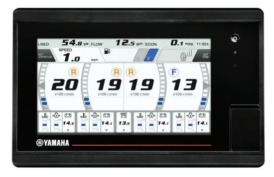
Yamaha Command Link CL7 Display (Digital Engines & Helm Master™)
