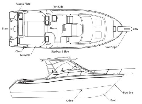
Abeam: a line perpendicular to a boat's keel
