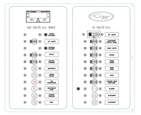
120V AC presents a high voltage shock hazard. All power supplies should be turned off and disconnected before accessing the wiring behind the AC panel. Service to the AC wiring should be performed by a qualified marine electrician.
