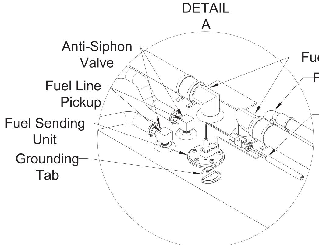
Fuel Fill Fuel Tank Vent Fuel Tank Harness
