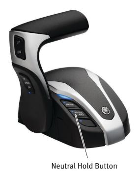
With the Helm Master EX<sup>TM</sup> system there is a feature that is similar to a neutral hold on other boats. When activated, the neutral hold button allows opening the throttles on all engines without engaging the forward or reverse gear. The active indicator will be illuminated during operation.
