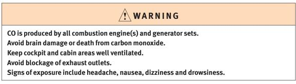
Carbon Monoxide, commonly written CO, is a colorless, odorless gas emitted from any boat's exhaust. The gas is similar in weight to the air we breathe. Therefore, it cannot be expected to rise or fall, but will accumulate in confined spaces.
